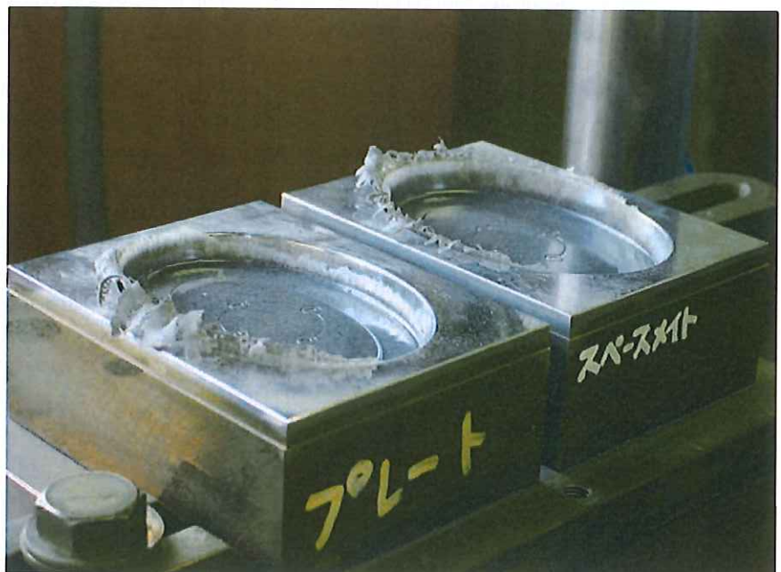
An extremely hot product immediately after compression molding at high temperature.
